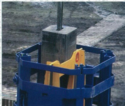
Modular drop mass placed in container
