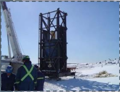
Statnamic catch mechanism at McMurray, Canada
