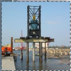
US 90 Biloxi Bay 24-in Statnamic Catch mechanism
