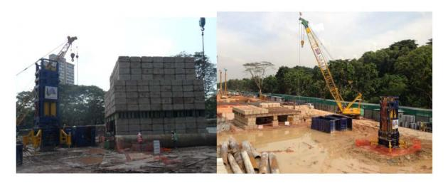
Quasi-Static Load Testing or a.k.a Rapid Load Testing (RLT), by which a quasi-static load is applied to a foundation test pile is used increasingly as an alternative to Static Load Testing around the world.
